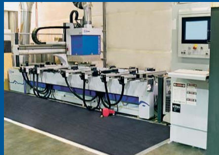
Work surfaces are meticulously crafted to your specifications using our highly accurate computerized equipment. A 3mm edge banding is applied all the way around the surface.
