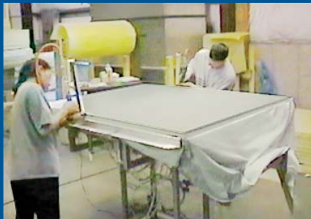
Our panel department covers over 350 panels daily. Fabric is applied and newly sanded and painted shells are installed along with a reused hanger rail and a new top cap.
