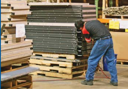
When a shipment arrives hardware is removed from all panels, shelves, and work surfaces. Each component is carefully inspected and reconditioned as needed.
